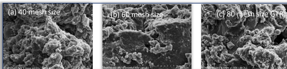
Figure 1(a-c). SEM micrographs of the GTR used for the work
