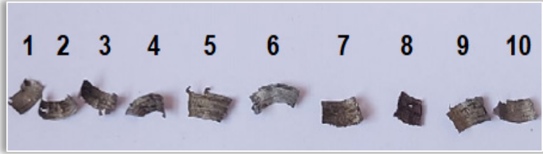
Figure 6. Measurements carried out for the determination of chip thickness in Experiment 1
