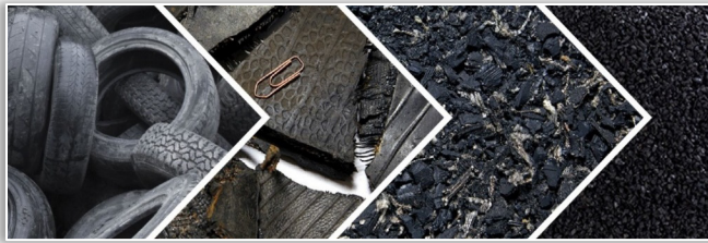
Figure 3 Tires—Tire shreds—Rubber chips—Rubber granules
