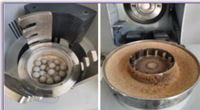
Figure 2. Size reduction of the material using a ball mill and an ultracentrifugal mill
