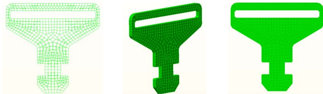
Fig.9. Discretization (meshing) of the latch plate model
