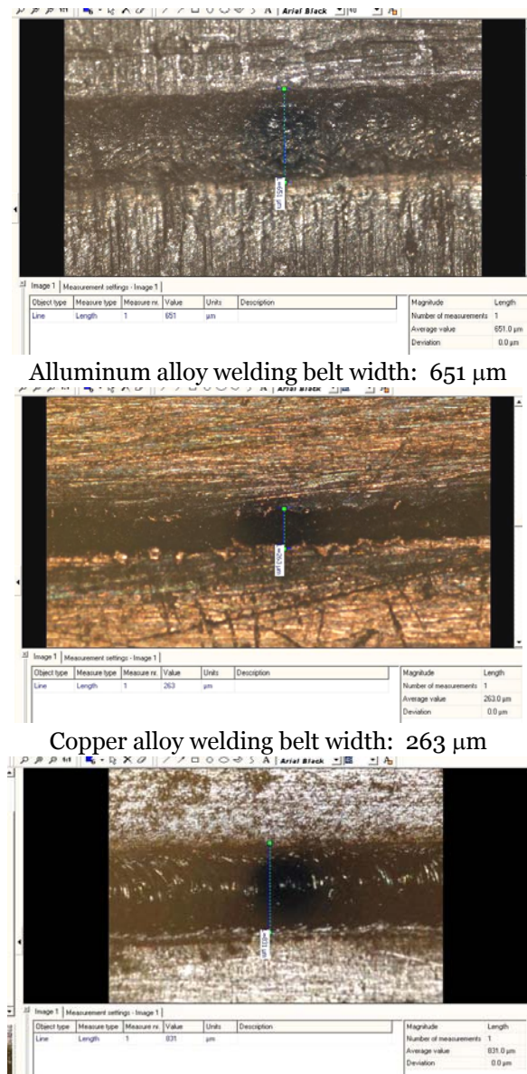
Fig. 8. Microscope images of the welding belts
