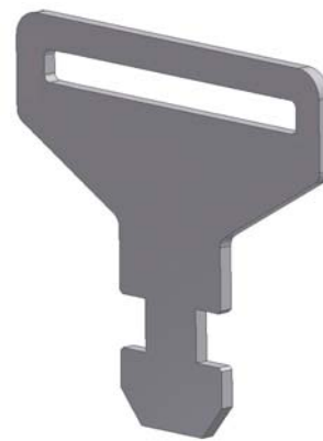
Fig.8. Geometric parameters and the 3-D model of the latch plate
