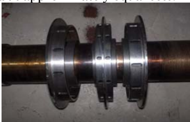
Fig.5 Lateral and intermediate support discs provided with channels mounted on the main axis, prepared for sample mounting
