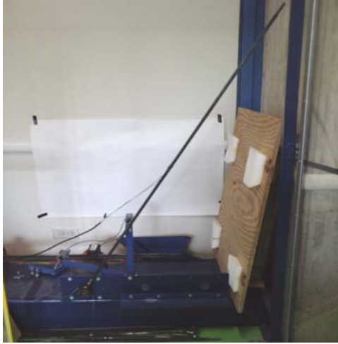
Figure 3: The flexible-link mechanism used for experimental tests
