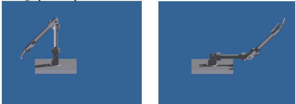
Figure 2. A 5 DOF robot arm with Angle1 and Angle2 parametres at the shoulder and elbow articulations were identified for the control VBA Macro program
