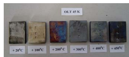
Figure 3. Lot samples OLT 45K, unused material, tested at high temperatures
