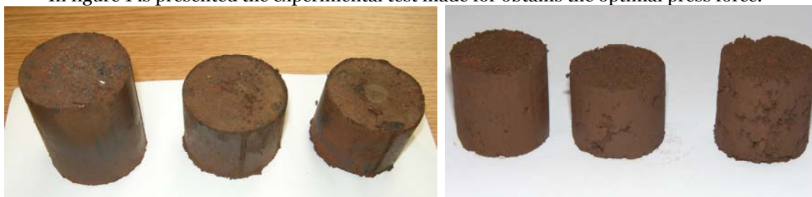
Fig.2 Experimental briquette made with hydraulic press and manual installation
