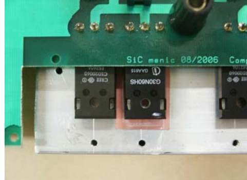
Figure 9. Detail of hybrid VSI devices
