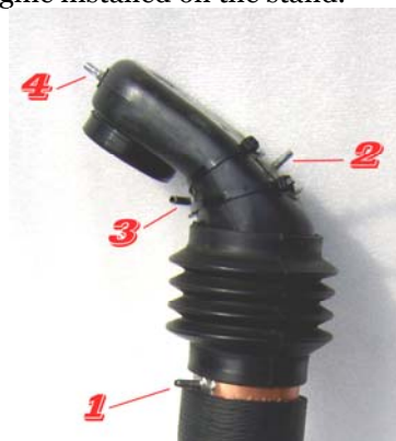
Fig. 2. Placement and numbering of the pressure plugs
