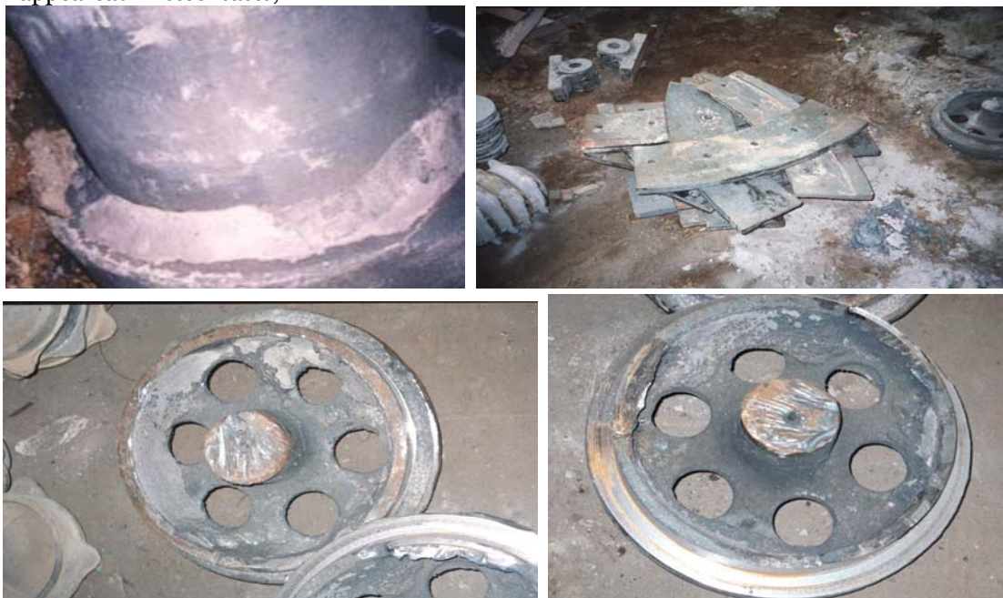
Figure 3. Castings presenting non-metallic inclusions and adherences. Cavities, micro-cavities and pores (B 311) appeared at a rate of 3,59%;
