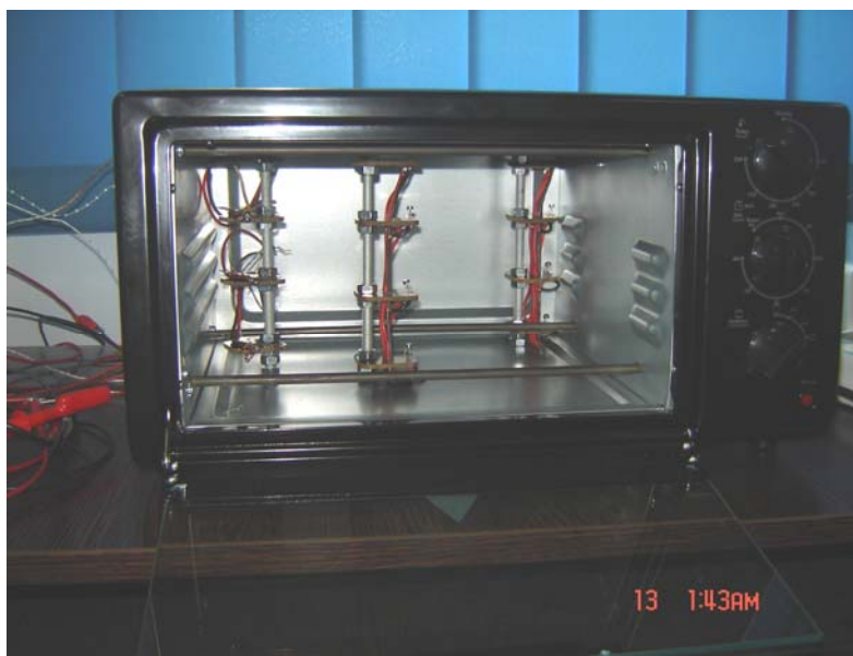
Fig. 2 Placing of the 8 sensors LM35DH inside the resistance oven
