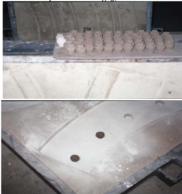
Figure 6. Mould cores made to obtain the holes of the casting Armor and fitting them into the mold.
