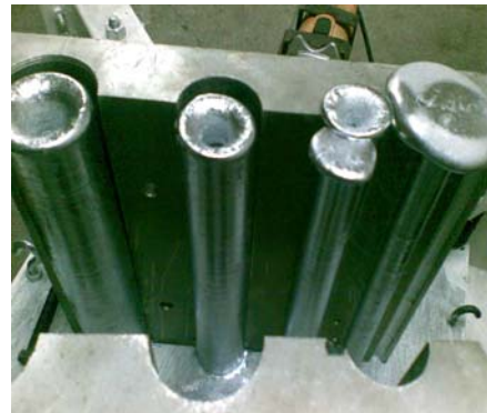
Fig. 2 Extraction of vibrated samples from the mold
