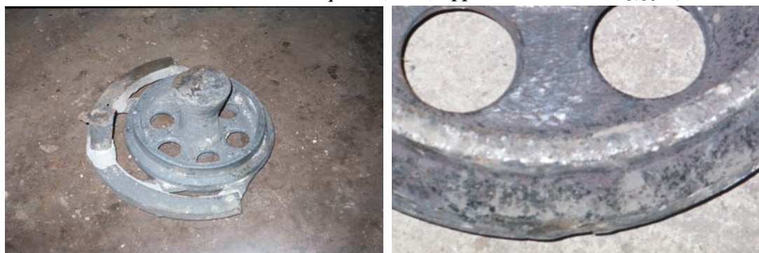
Figure 4. Casting presenting micro-cavities and pores.
