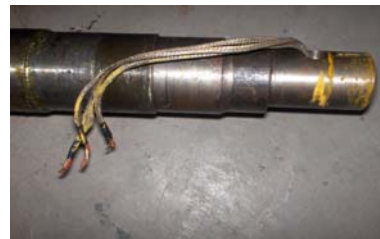
Fig.6 Thermocouples crossed through the main axis of the facility to connect their data acquisition system
