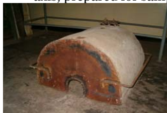
a - overview of the oven for sample heating
