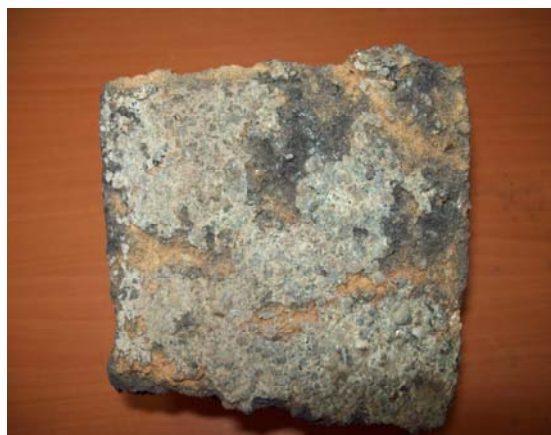
Fig.2. Interface between slag layer and brick
