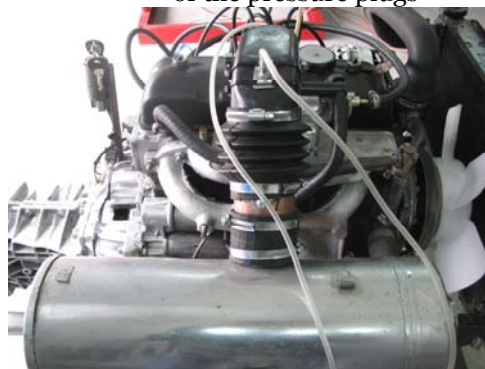
Fig. 4. Stand trial of the original classic filter
