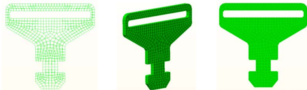
Fig.9. Discretization (meshing) of the latch plate model
