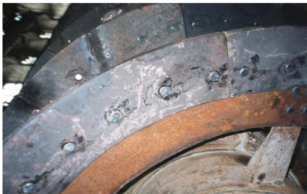
Figure 10. The armor mounted on spiral classifier
