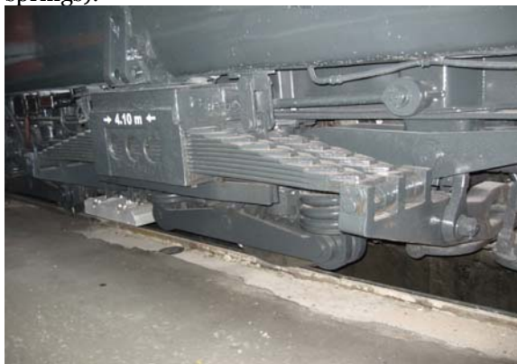
Fig. 1: Bogie with leaf spring
