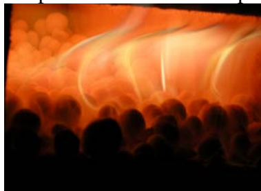
b. Burning pellets in volatile release and clearance of carbon monoxide
