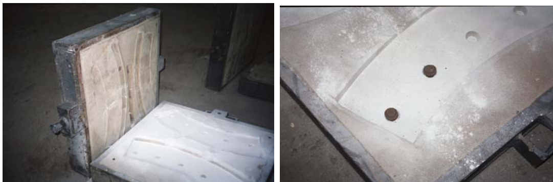
Figure 9. The mould parts (upper and lower), before assembly for casting.
