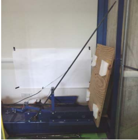
Figure 3: The flexible-link mechanism used for experimental tests
