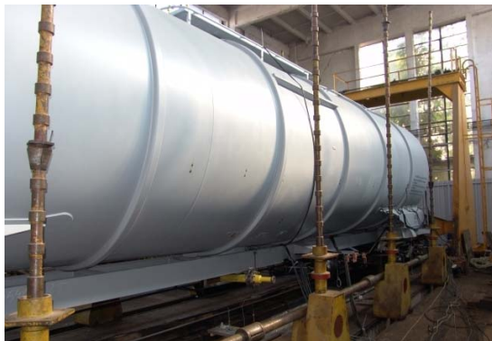
Fig. 1. The tank wagon on AFER's Stress Analysis Bench Test
