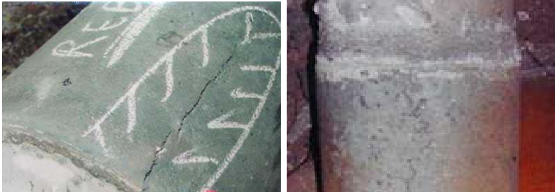
Figure 5. Castings presenting fissures.
