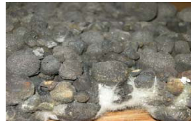
a. pellets heated at a temperature of 1050 oC respectively 1250 oC
