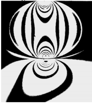
Fig. 4. The isochrones photos for R_1/R_2 = 0,58 at q=74,21 N/mm, the higher level of isochrone n=8 \varphi_0
