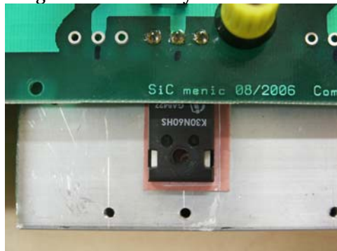
Figure 11. Detail of VSI with classical device
