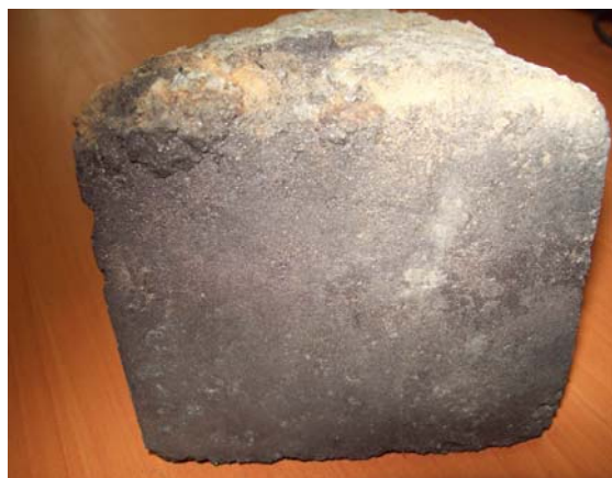
Fig.1. Deposited slag on brick after its used in LF
