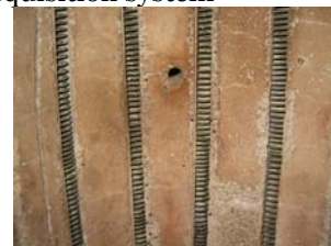
c - loop mounting resistors for electric sample heating oven
