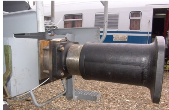
Fig. 8. Load cell mounted under the buffer
