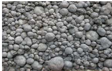
a. pellets heated at a temperature of 1050 oC respectively 1250 oC
