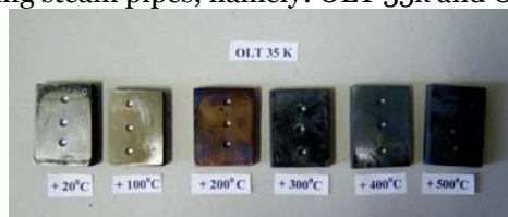
Figure 2. Lot samples OLT 35k, unused material, tested at high temperatures
