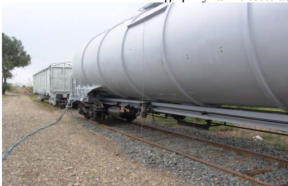
Fig. 5. The tested wagon and the ramming wagon
