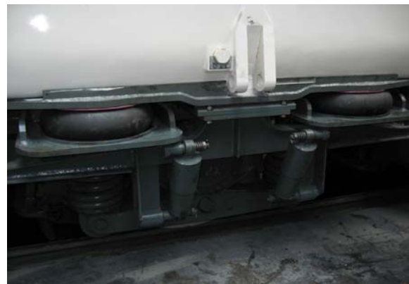
Fig. 2: Bogie with rubber spring
