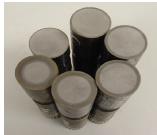
Fig. 2. Some pieces with different hardening depth depending of generator power, frequency and maintained time in inductor
