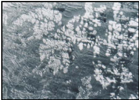
Fig. 1.9. Table R1 ceramic impregnated with copper zone of transition between the coated and impregnated; 250X
