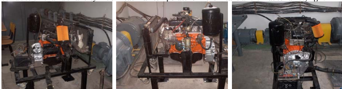
Fig.1 The experimental bench with ignition engine type Dacia
