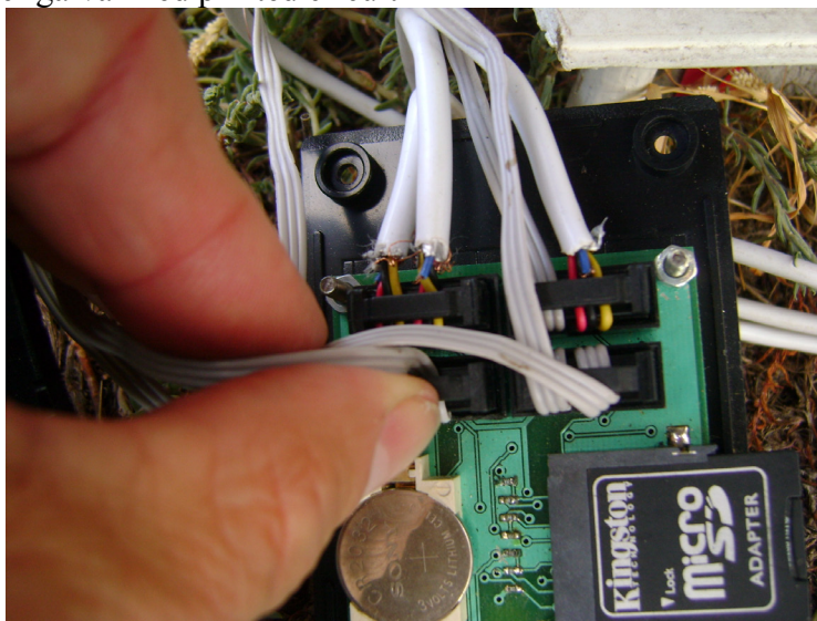
Figure 4 - PIC18F4550 type micro controller unit with wires, SD memory card and CR2032 battery for the clock.
