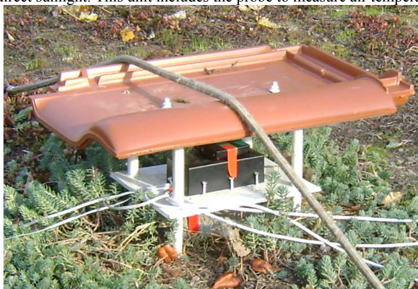
Figure 3 - Electronical unit with weather protection, battery, and wires
