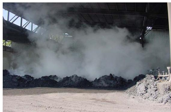
Figure 4. Cooling area with water spraying
