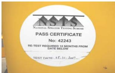
Figure 8. Plaquette for periodic verification of the pest and deseases control equipment in England.(Photo Bungescu England 2008)
