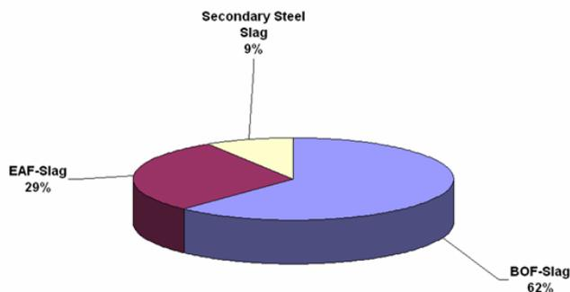
Figure 1. Type of steel slag
