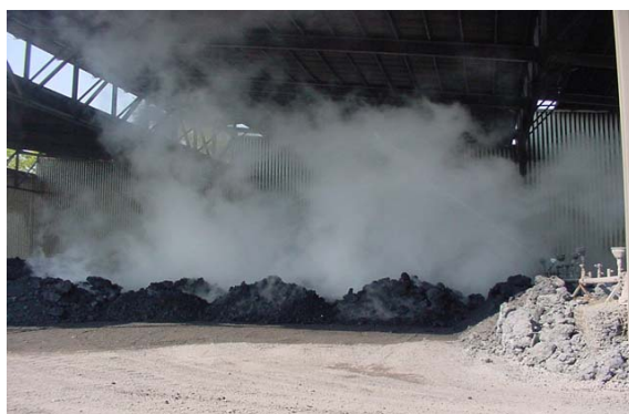
Figure 4. Cooling area with water spraying
