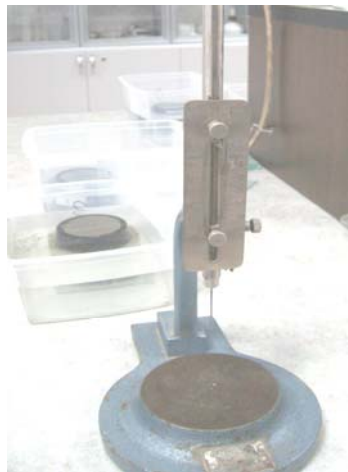
Figure 10. Vicat apparatus for determination of water for the normal consistence paste and resulting proofs.
