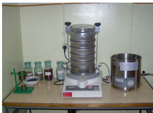
Fig.4 The screening installation „Analysette 3” Fritsch, the grain size 25 \mu m - 2 mm
