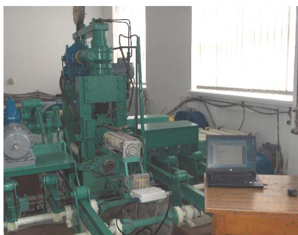
Figure 4. The assembly of experimental rolling mill
