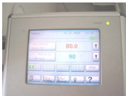
Figure 1. Control and monitoring panel for climatic chamber Vötsch, type VC 7060
