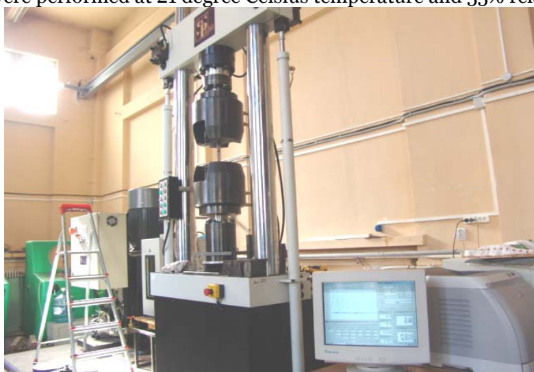
Figure 1 The Universal Testing Machine SI-PLAN 942-1 type
