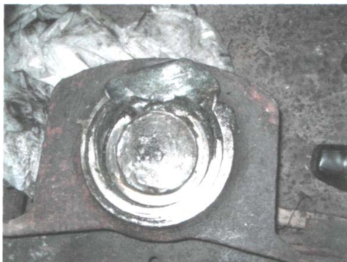
Figure 2. The aspect of the fracture zone in the extremity of the wheelset (lubrication boxes)
