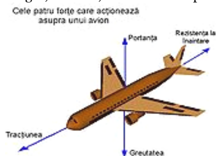
Fig 1 Force systems which operate on an airplane
