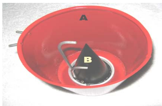
Figure 9. The external axial collector with the internal cone (radial view)
