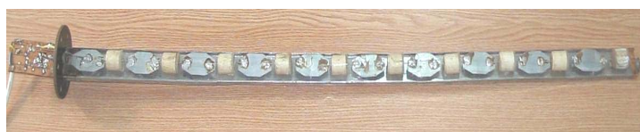
Figure 3. The resistive transducer used in experiments
