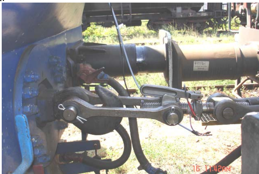
Figure 2 Drawing hook with strain gauges
