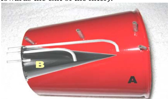
Figure 8. The external axial collector with the internal cone (longitudinal view)
