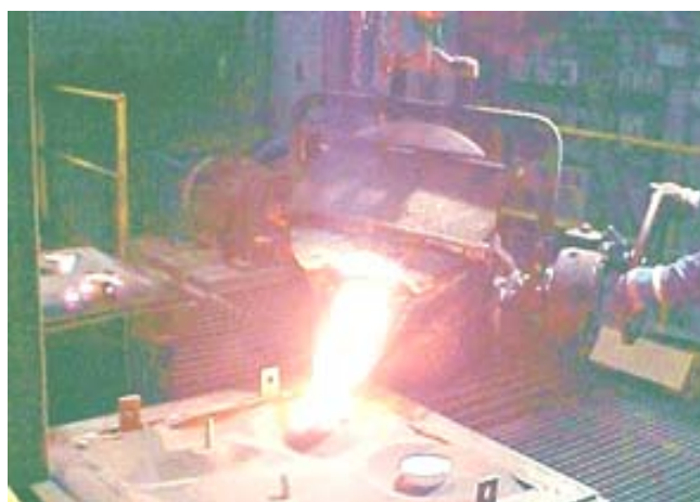
Figure 1. An electromagnetic pump for casting melted cast-iron
