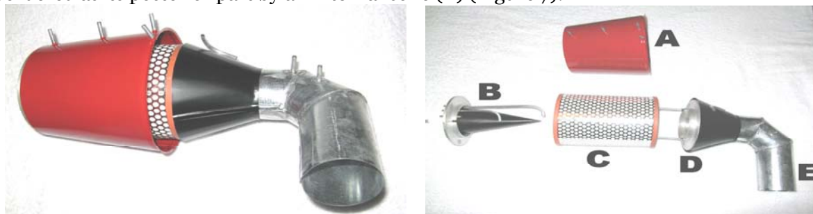
Figure 7. Inverted super-absorbing filter. Constituting elements
