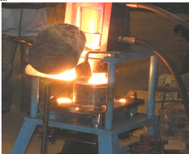
Figure2. Casting of the melt in the die
