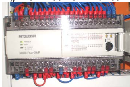
Figure 6. PLC of device for checking plain bearings
