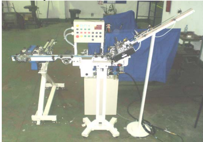
Figure 5 Device for checking plain bearings
