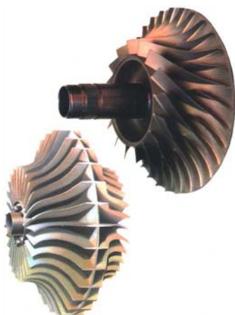
Fig. 2 Specific constructions of rotors of centrifugal compressors in aviation
