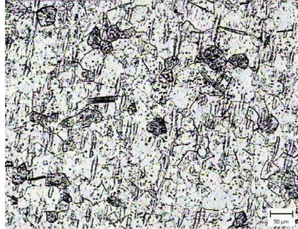
Figure 2. Titanium alloy substrate BM (cupric solution, 100 x)
